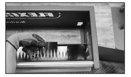
4. While clamp bar is still locked, cut off excess belt from first section of punched fingers, unclamp, and shift the belt to the left.
