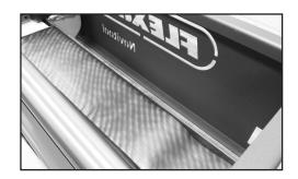
9. (Belt End 2) With the edge of top cover against the c-clamp tray belt stop, fold bottom cover back clamping it between the clamp bar.
