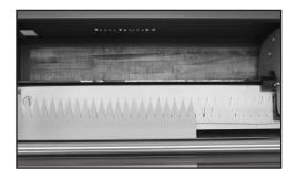
15. Prior to re-clamping and resuming punch process, measure the distance between the leading belt edge and the c-clamp tray stop on the left, and be sure the distance measures the same on the right leading belt edge prior to clamping and resuming punch process. Repeat process until the entire belt end has been punched. NOTE: Be sure none of the fingers are out of alignment underneath top cover prior to resuming punch process.
