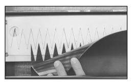
7. Prior to punching the top cover, release the clamp bar allowing the top cover to lay over the already punched fingers. Line up the left edge of the top cover with the peak on the left side of the punch board making sure the front edge of the top cover is up against the c-clamp tray belt stop and lock in place. Slide and lock the PUN M<sup>™</sup> tray in the back position and resume the punch process until you've utilized the complete cutting surface of the punch board.
