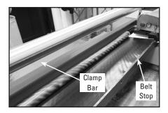
**2.** (Belt End 1) With the edge of the bottom cover against the c-clamp tray belt stop, fold top cover back clamping it between the clamp bar.
