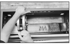
10. Begin punching the top cover by following instructions starting on pg.19 of the PUN M<sup>™</sup> Manual Finger Punch Safety and Operation Manual until you've utilized the complete cutting surface of the punch board.
